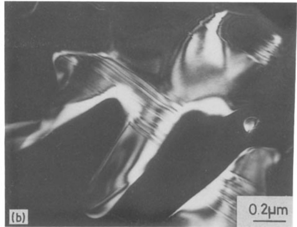
Figure 16 (a) BF and (b) CDF images of a crystalline intergranular phase in a \text{Si}_3\text{N}_4 + 20 \text{ wt } \% \text{ Y}_2\text{O}_3 + 2 \text{ wt } \% \text{ Al}_2\text{O}_3 specimen after sintering at 1800^\circ\text{C} for 4 h in nitrogen. An EDS analysis obtained from that area is given (c).
