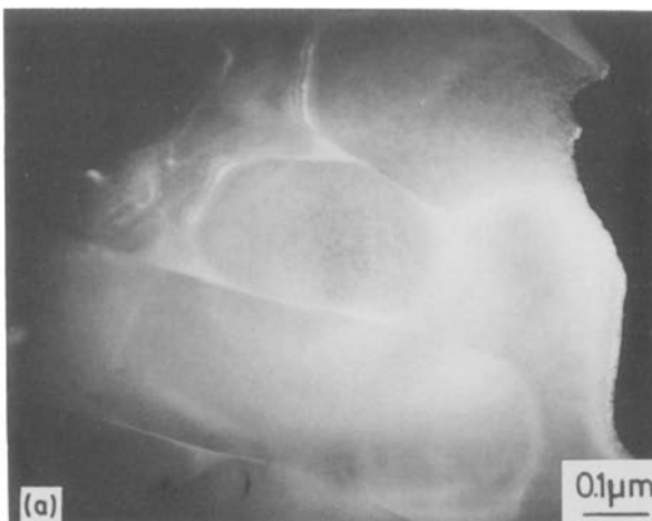
Figure 17 (a) CDF image of the vitreous intergranular phase and (b) direct lattice image of a \beta -silicon nitride grain.
